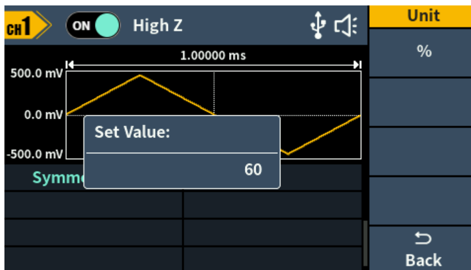
Figure 5-6: Set the symmetry of ramp wave
